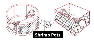
A shrimp pot with no definable sides, such as a round pot, must have 50% of its vertical surface area covered with 7%-inch webbing. The other 50% of its vertical sides, as well as its top and bottom, may be composed of any material
