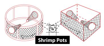
A shrimp pot with no definable sides, such as a round pot, must have 50% of its vertical surface area covered with  $\frac{7}{8}$ -inch webbing. The other 50% of its vertical sides, as well as its top and bottom, may be composed of any material
