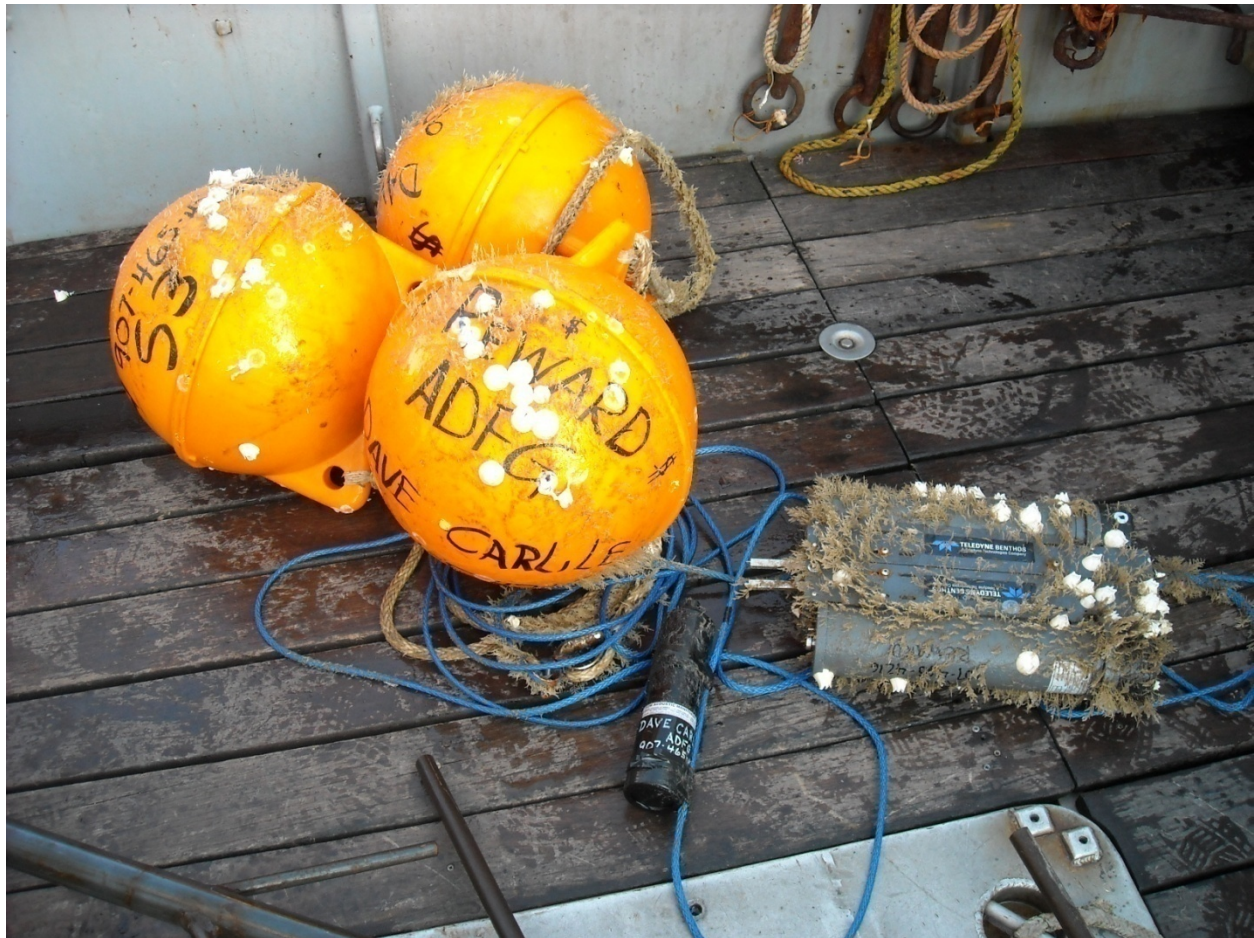
Figure 2. Trawl floats, acoustic receiver, acoustic releases and tether line (blue) from acoustic subsurface mooring retrieved by dragging with grappling hook.
