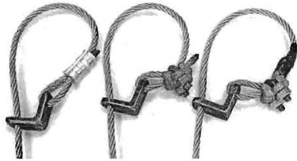
Fig. 7. Most reliable foot loop configurations for withstanding forces >16.8 kN. Left: aluminum sleeve; middle: dead horse Crosby® clip; right: live horse Crosby® clip.
