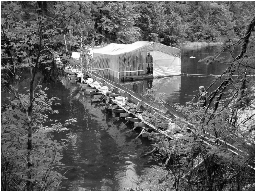
Figure 6.—View showing the adult picket weir with attached trap and covered sampling raft located at the outlet of Slippery Lake.
