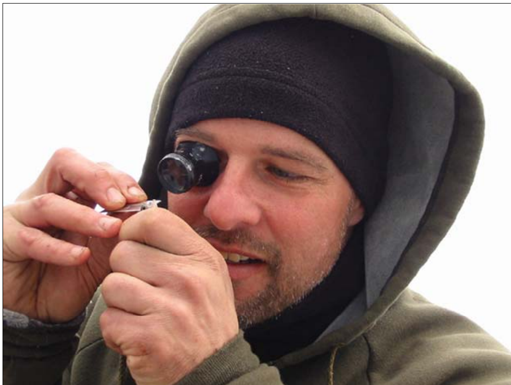
Figure 42. —Checking tag placement with jewelers loupe and single edge razorblade.
