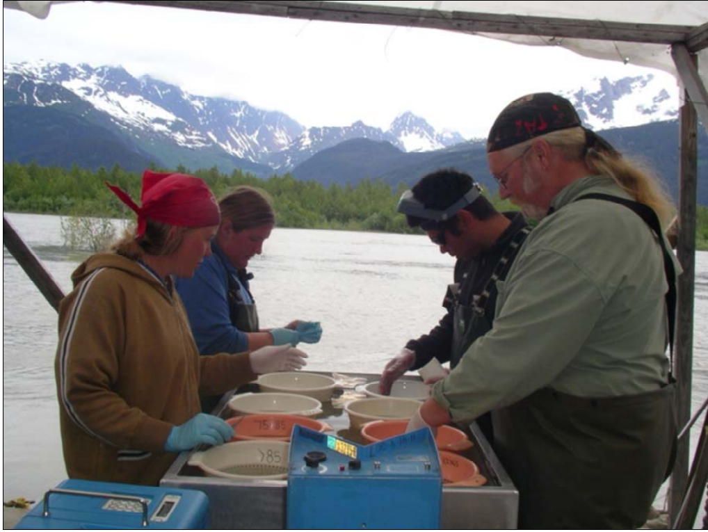
Figure 39. —Sorting and clipping set up at Taku river smolt camp. Note water table and colanders labeled for sorting fish by size. Water table contains MS222 solution. River water is pumped through copper tubes in the water table to keep the water cool.
