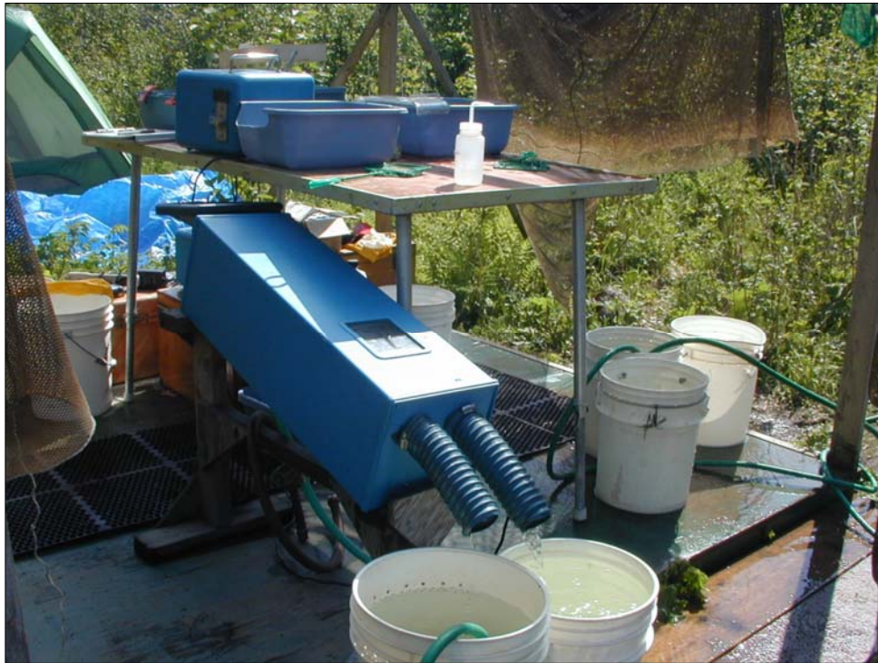
Figure 31. —A Quality Control Device is included in this tagging operation. Hoses are used to refresh fish holding buckets. The buckets are modified with drain holes. Also note the use of rubber foot relief mats and the cut-down side of the tagging pan.
