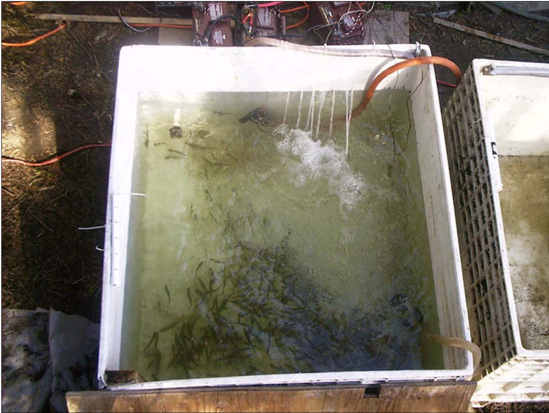
Figure 29. —On-land fish holding box on the Chickamin River with aeration and 12 volt fresh water pump.
