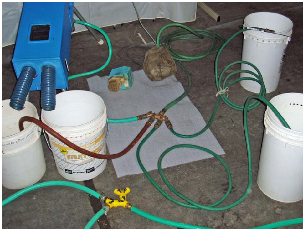
Figure 32. —QCD with submersible water pump and two examples of hose set ups and spill buckets.
