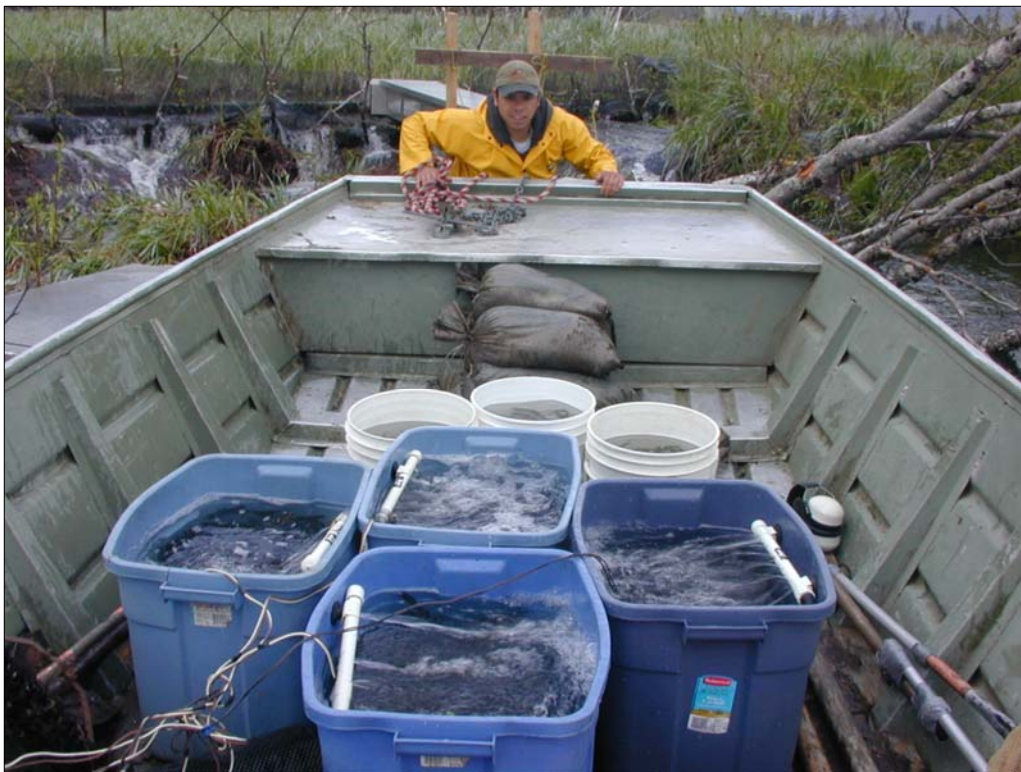
Figure 26. —Four aerators are powered by the 12V battery that is used to start the outboard motor. Buckets are also being used to hold fish. The totes are 18-gal size; they have long straight sides suitable for mounting the aerator spray tube. In the background is the dewatering trough of a spill trap installed in the outflow from a beaver dam.
