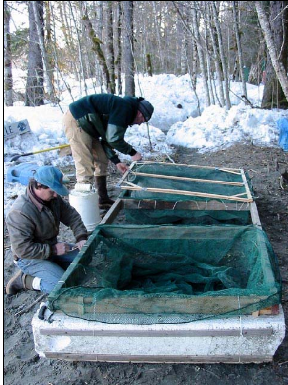
Figure 27. —Construction of floating net pens with Styrofoam floats. Note lid to keep out predators.
