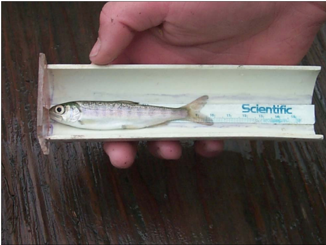
Figure 44. —Smolt measuring trough made from 2 in PVC plastic pipe.
