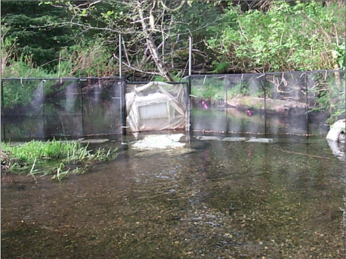
Figure 13. —Example of a simple Vexar® panel smolt weir on a tributary of the Nakwasina River.
