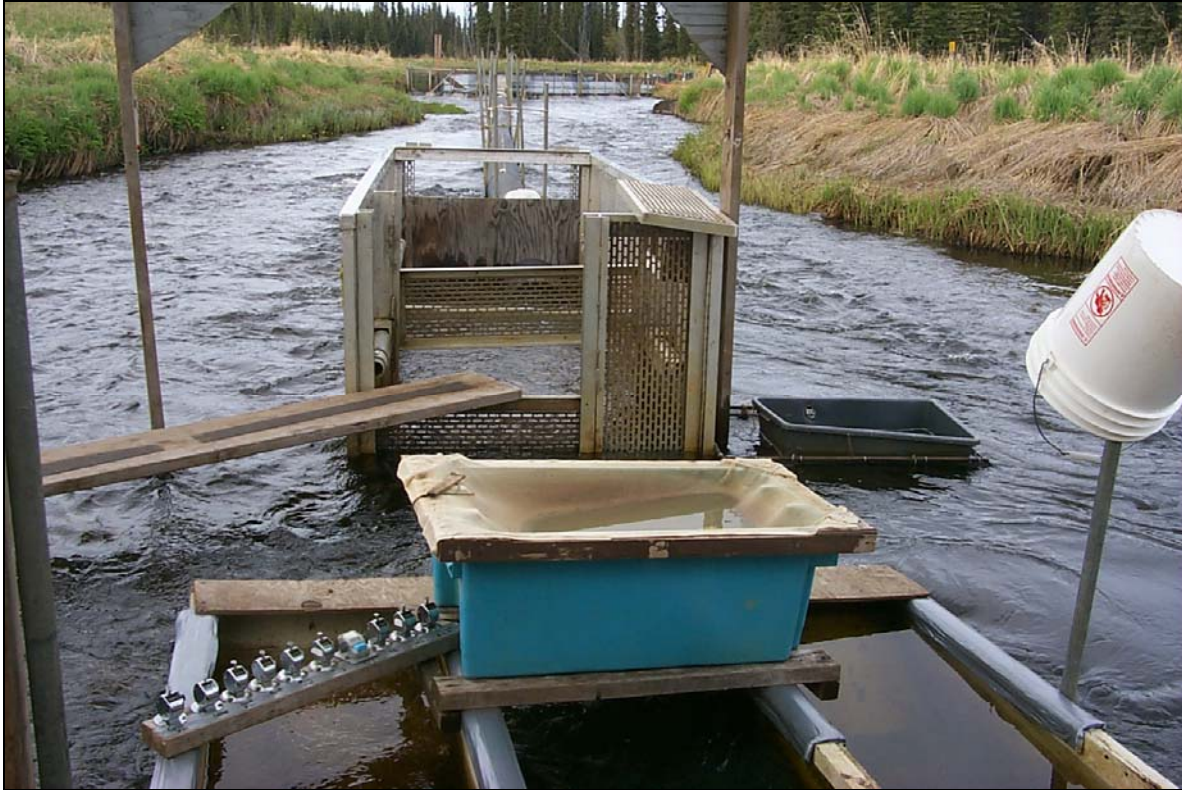
Figure 35. —The live box and sorting tub at Moose River smolt weir. Note moveable panels in live box and base mount talley counters for counting other species and upstream migrants.
