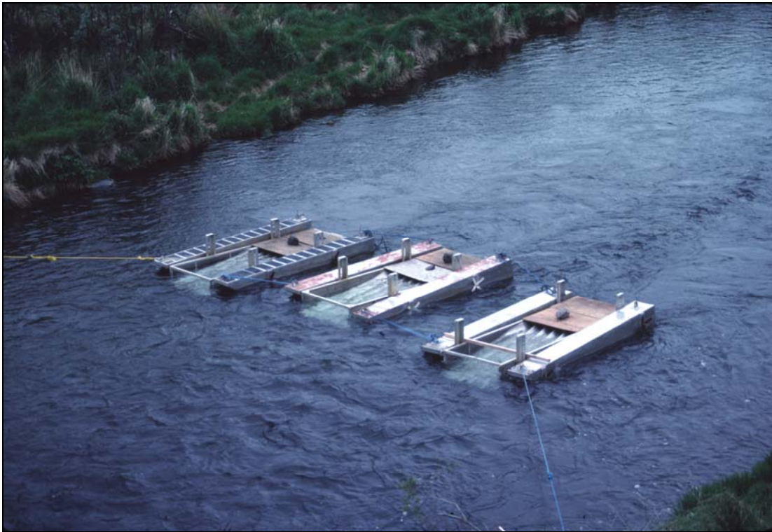
Figure 25. —A battery of inclined plane traps deployed on the Thumb River. Note cable hinders river navigation.
