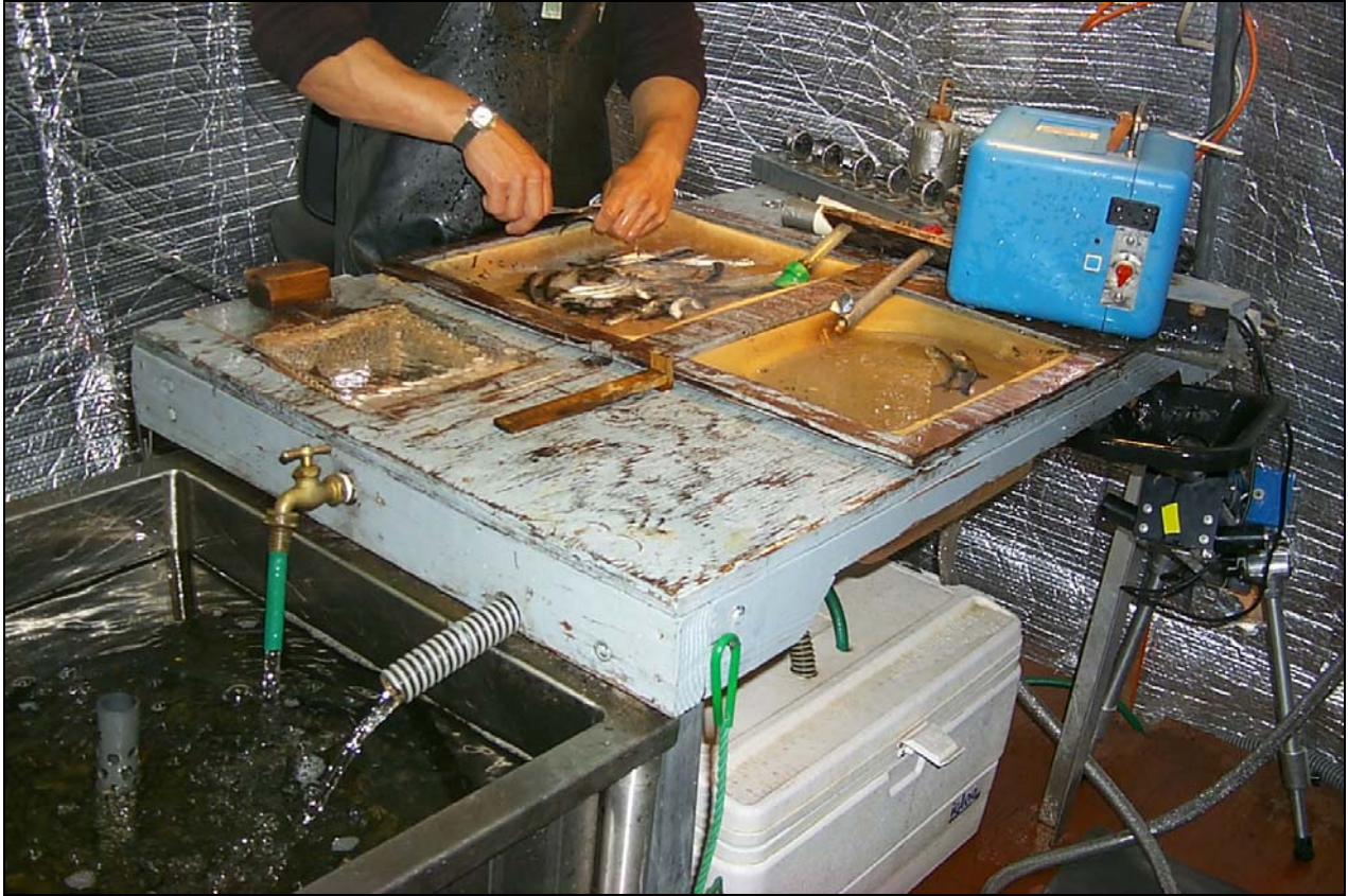
Figure 36. —Tagging table at Moose River weir. Note small tub with dip net of fish in it and plexiglass cover to keep them from jumping out. That tub and upper tub have MS222 solution pumped through them. Tub on the right has fresh water pumped through it. Stainless steel industrial sink with overflow tube is used to hold fish prior to tagging, fresh water pumped through it. Note cooler on floor contains the MS222 solution. Quality control device drops tagged fish directly into holding pens in the river for recovery.
