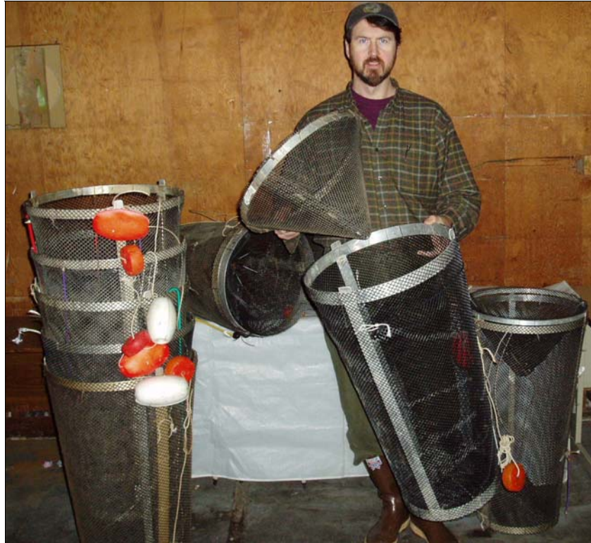
Figure 2. —Large stacking fish traps designed by Kent Crabtree. The large cone entrance is removed for easy access to the catch and for baiting.
