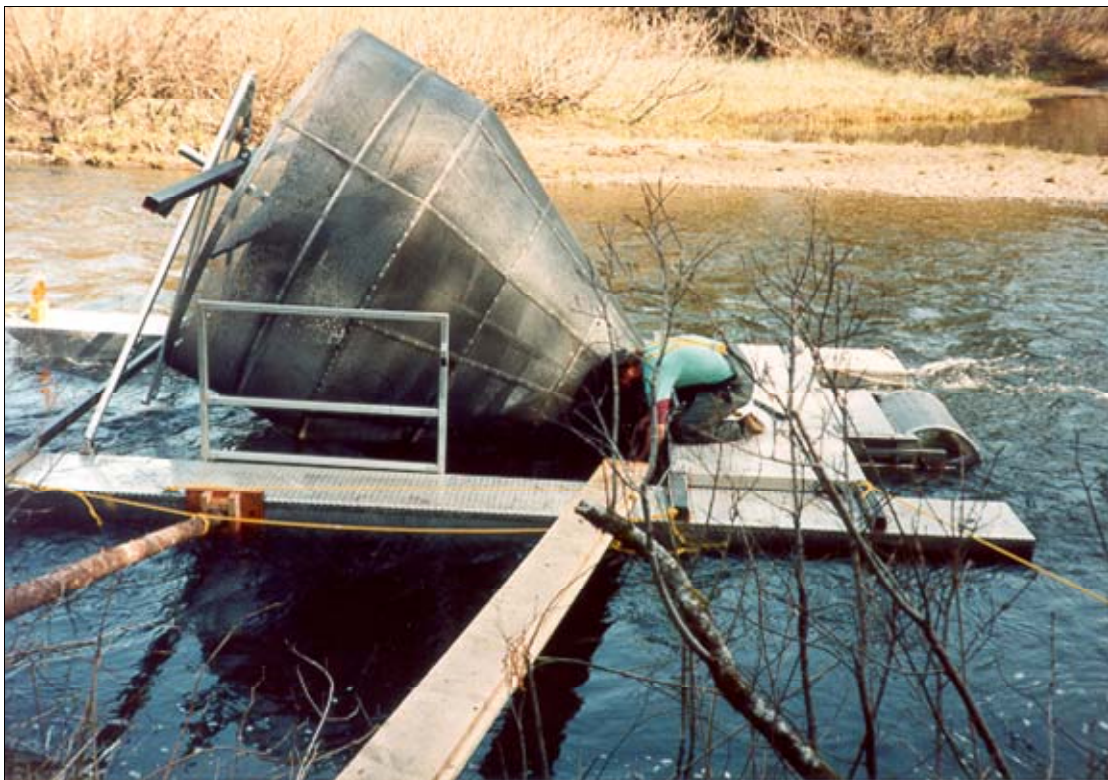
Figure 24. —Rotary screw trap raised from water for cleaning. Note boom log and safety light.
