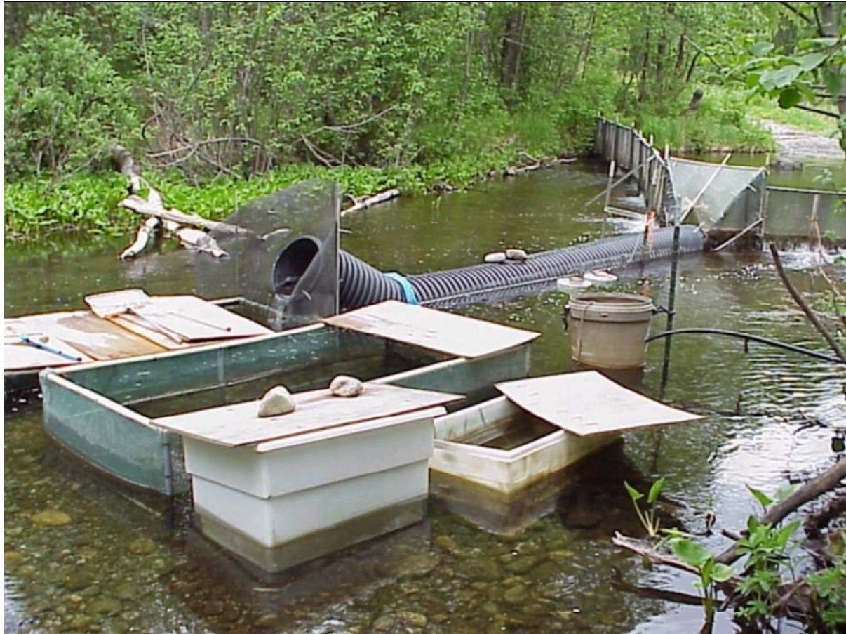
Figure 14. —Cottonwood Creek weir. The water level on the upstream side of the weir was higher than the downstream side and the tube had an acute upward bend. Debris on the weir served to dam the creek and, water flowed out the elevated tube only when the water level was high enough. The weir was cleaned only in the early evening and this temporarily dropped the water level and stopped the flow of water (and smolt) from the tube. Debris accumulated on the weir during the evening hours, and, by about 8 am, water was flowing from the tube again. This negated the need for around-the-clock crew shifts. The crew worked a normal day shift and one crew slept on site. Smolt occasionally attempted to jump from the trap back into the tube, so a funnel of Vexar® was placed around the discharge end of the tube to prevent smolt from missing the tube and landing in the creek.
