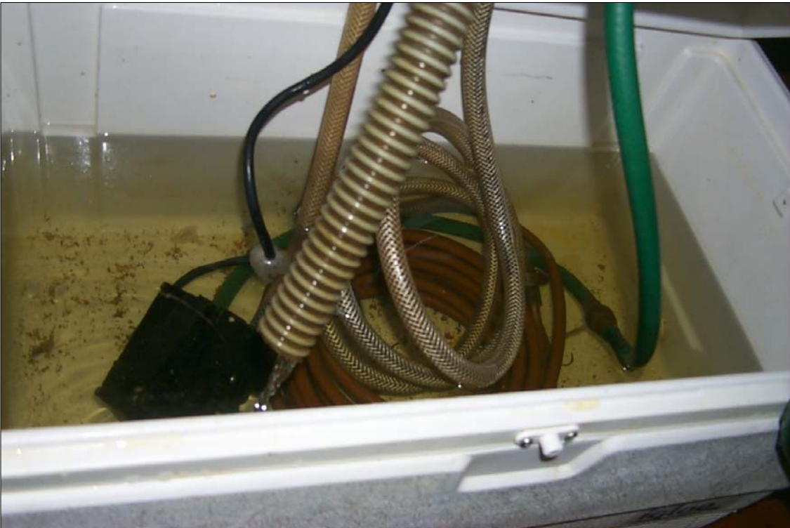
Figure 38. —Pump for recirculating MS222 solution and coil of copper tubing to circulate fresh river water through cooler to keep the MS solution from getting too warm.
