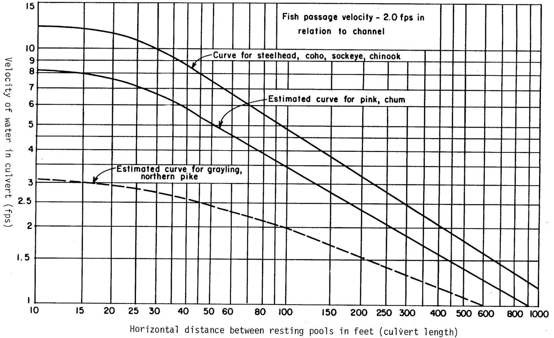
Figure 5-11. Swimming speeds of fish relative to horizontal distance between resting pools.
