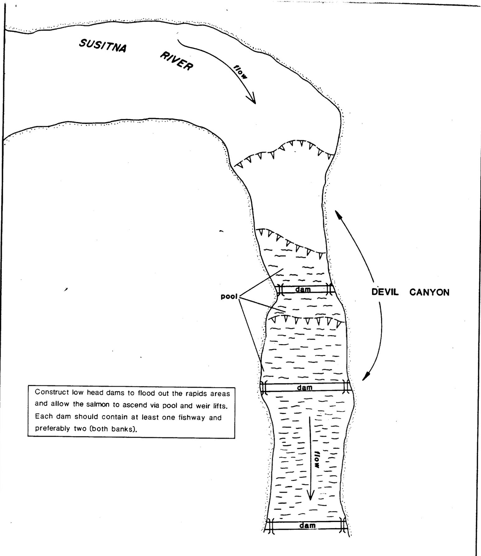
Construct low head dams to flood out the rapids areas and allow the salmon to ascend via pool and weir lifts. Each dam should contain at least one fishway and preferably two (both banks).
