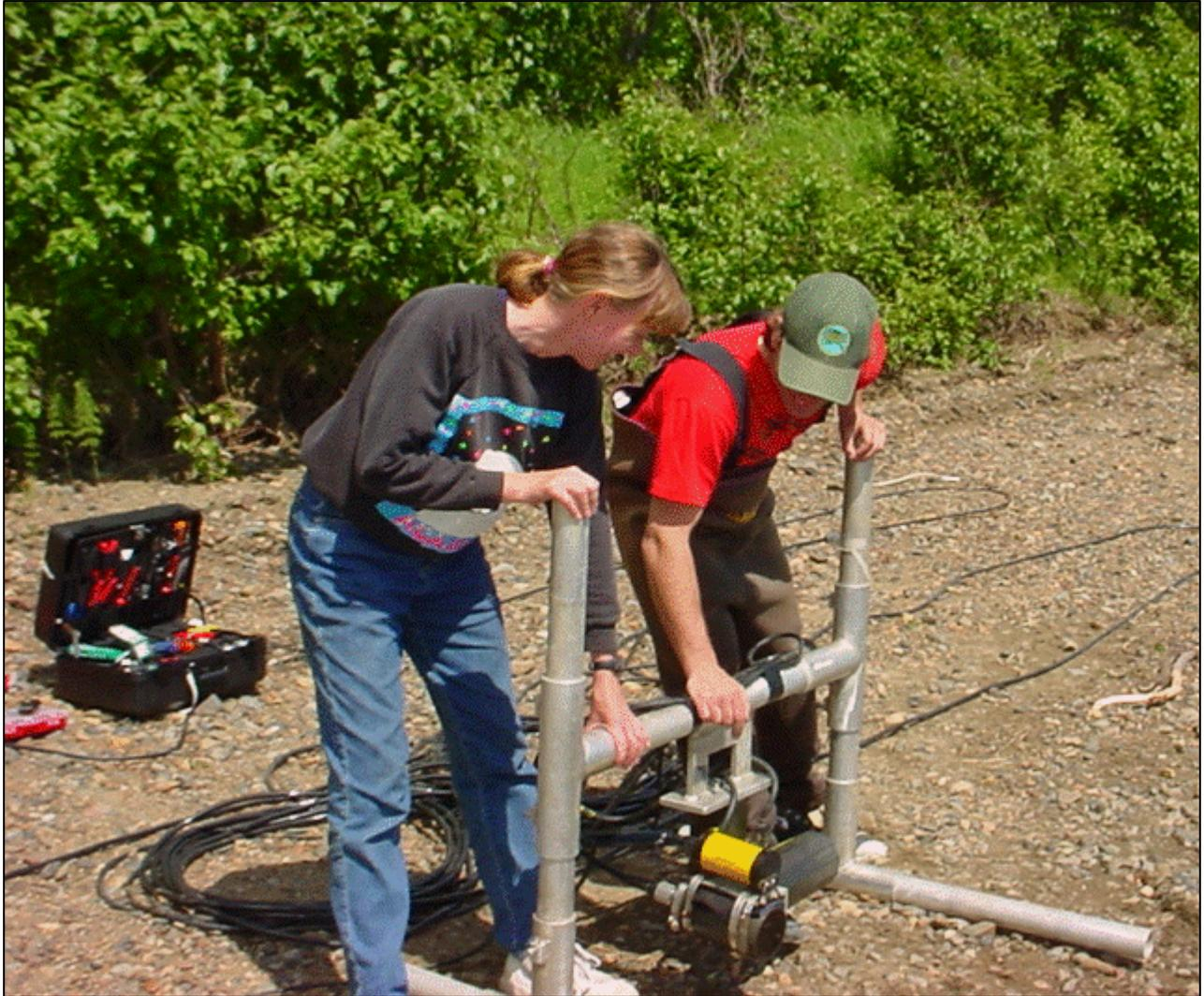
**Figure 2.**—H-mount made from aluminum poles with 2 single-axis rotators, a 4° by 10° HTI transducer, and a BioSonics' attitude sensor.
