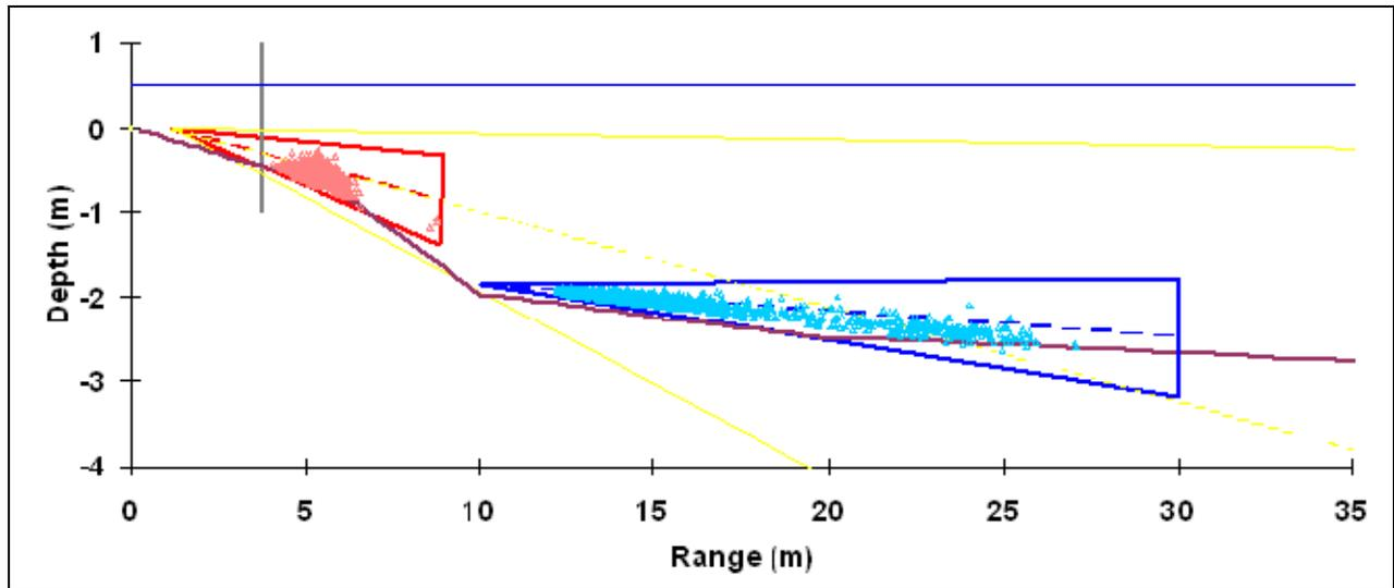
*Note:* The overlaid gray beam shows the potential coverage of a DIDSON 14° beam.
