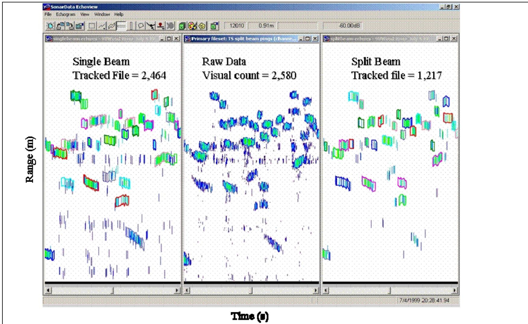
*Note:* A visual count of the complete data file resulted in 2,580 targets from the raw data, 2,464 targets from the single beam processed data, and 1,217 targets from the split beam processed data.
