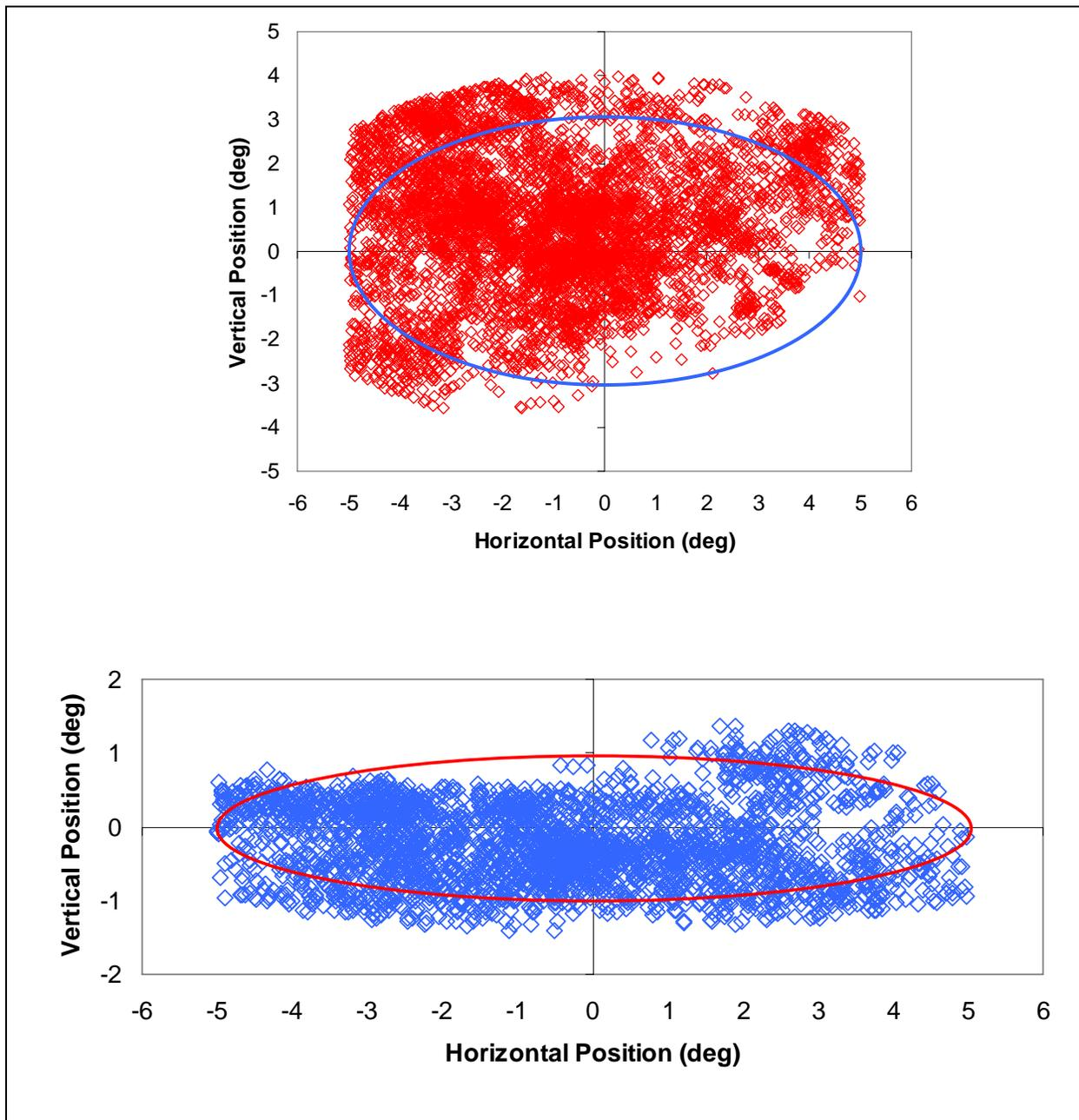
**Figure 12.**—The horizontal and vertical position of echoes reflected from the 38.1 mm tungsten carbide sphere with the nominal beams overlaid during calibration of the 6° by 10° (top) and 2° by 10° (bottom) transducers, Nushagak River sonar, 2003.
