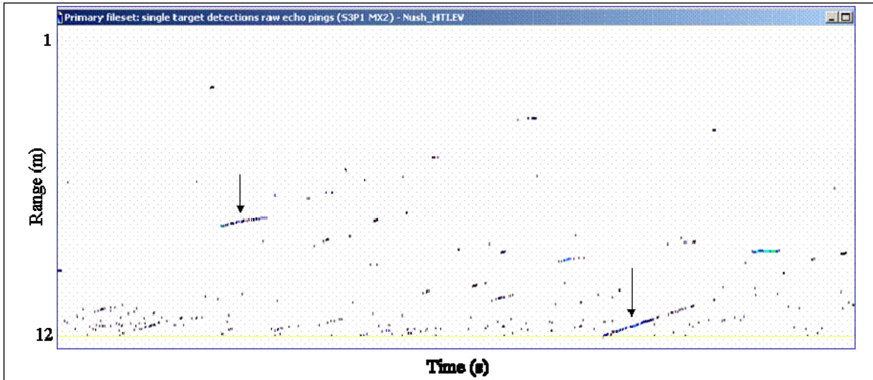
**Figure 29.**—An echogram from the offshore transducer with arrows pointing to traces from floating plant material, June 30, 2002.
