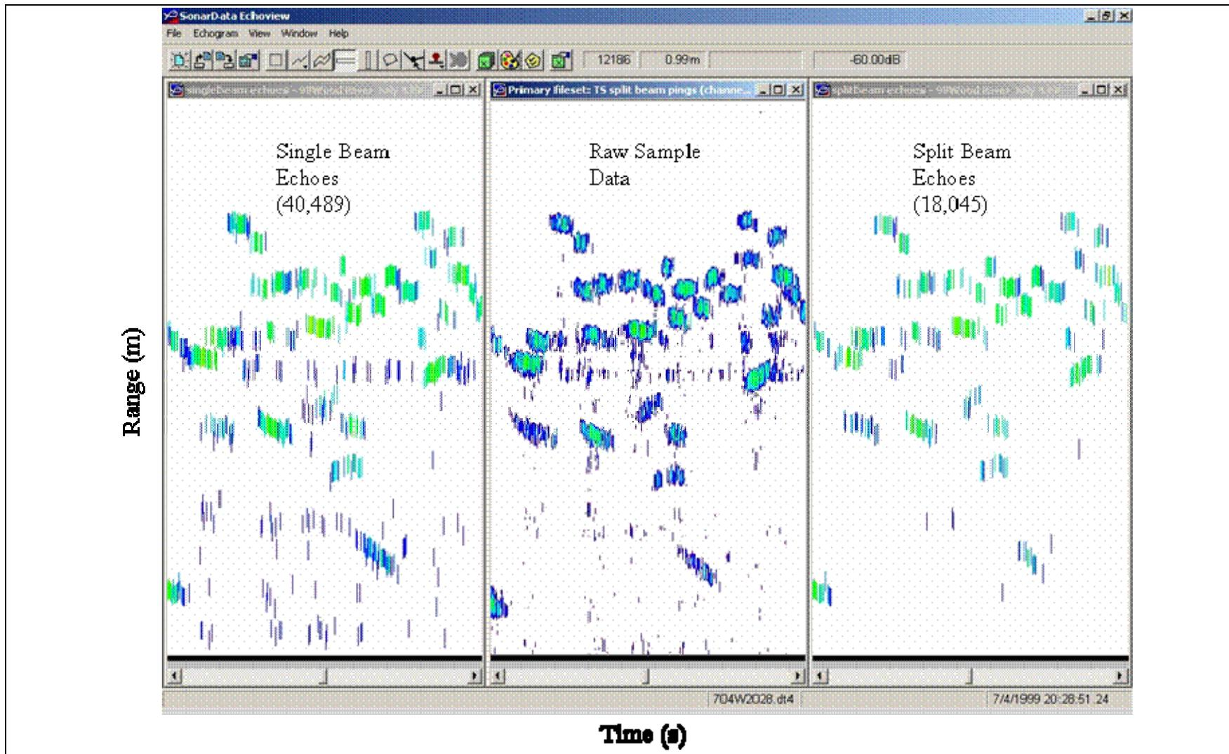
*Note:* The echo data results in far fewer echoes with the split beam processing when compared to single beam processing. Displayed with SonarData's Echoview software.
