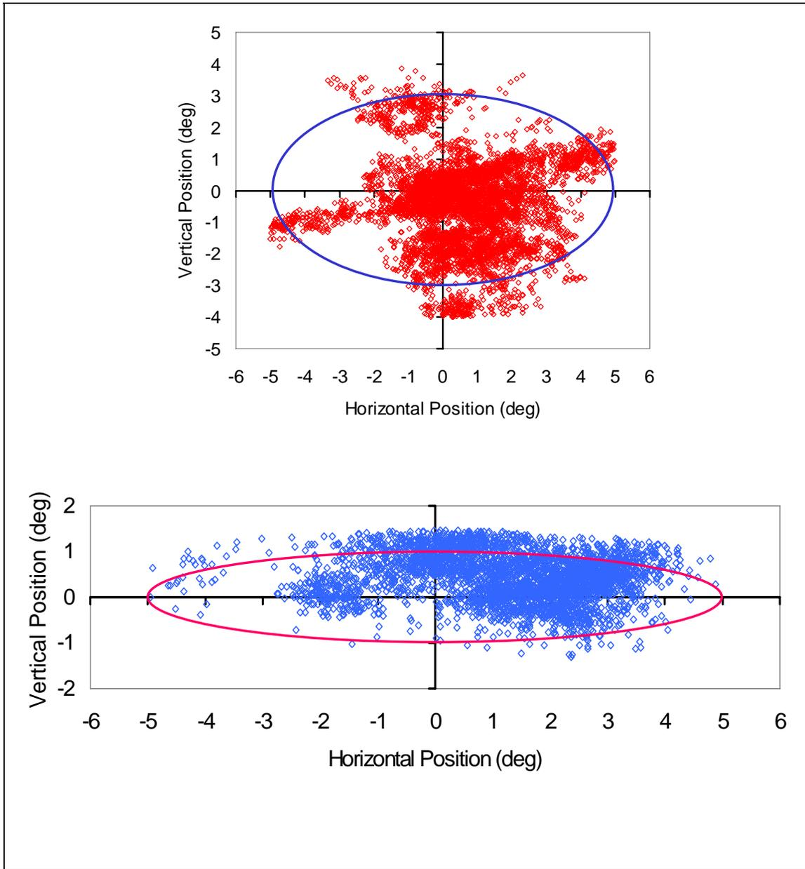
**Figure 11.**—The horizontal and vertical position of echoes reflected from the 38.1 mm tungsten carbide sphere with the nominal beams overlaid during calibration of the 6° by 10° (top) and 2° by 10° (bottom) transducers, Nushagak River sonar, 2002.
