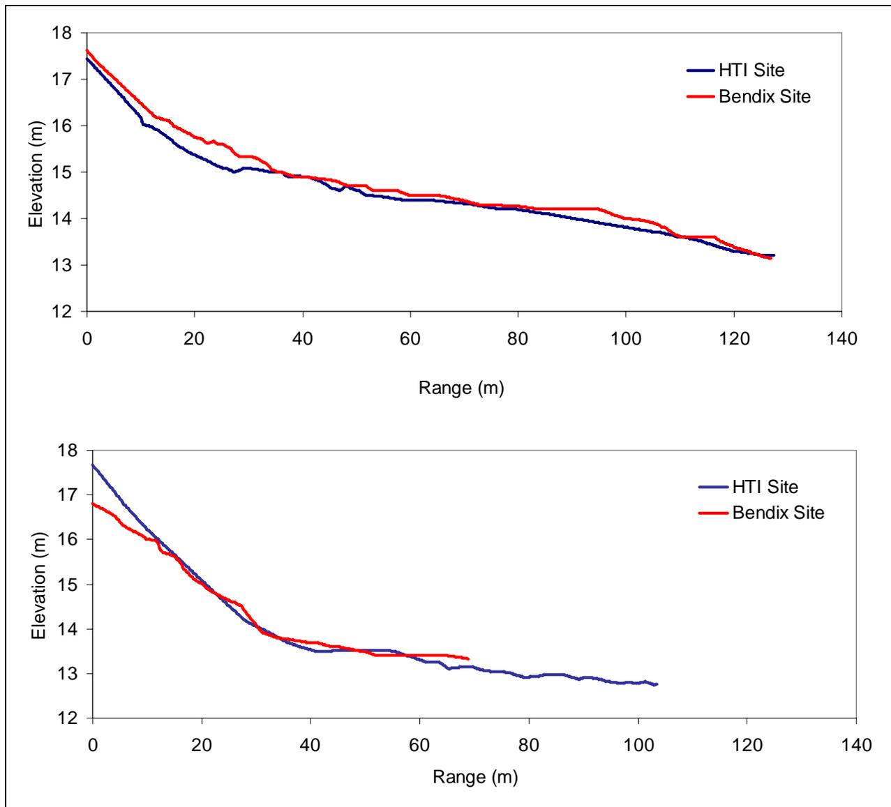
**Figure 9.**—River bottom profiles along the right bank (top) and left bank (bottom) of the Nushagak River at the deployment sites of the Bendix and HTI split beam sonars.
