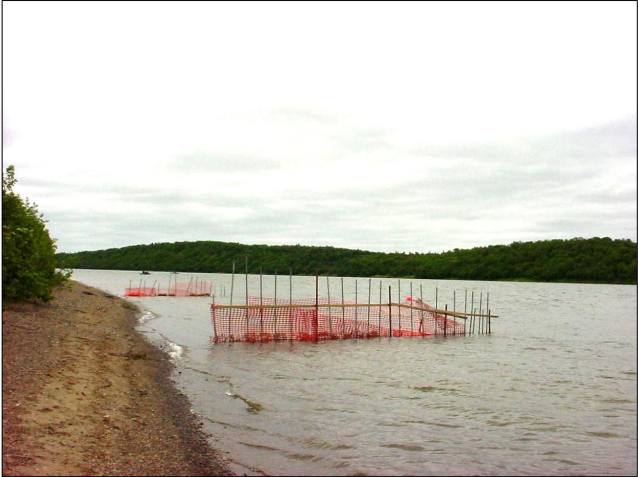
**Figure 3.**—Two weirs along the right bank of the Nushagak River for the Bendix nearshore transducer (foreground) and the HTI system (upstream), Nushagak River sonar, 2002.
