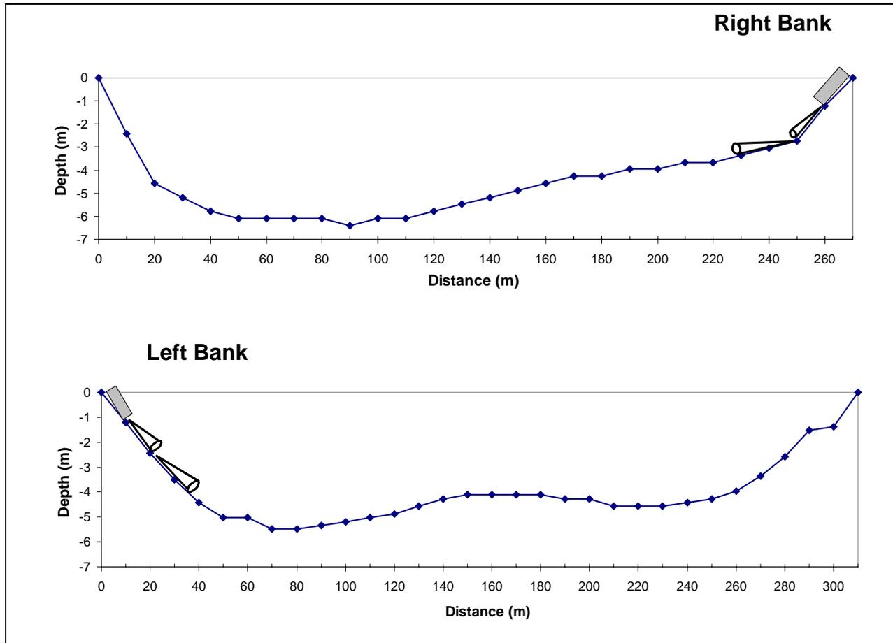
**Figure 5.**—Cross-river profiles at the right bank Bendix transducer site (top) and the left bank site (bottom) showing the approximate placement of the nearshore and offshore Bendix transducers, Nushagak River sonar site, June 10, 1999.
