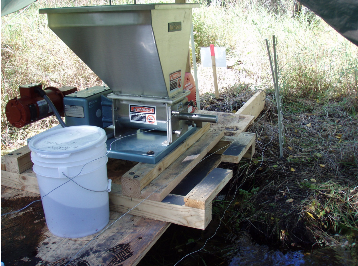
Figure 9.–Rotenone deactivation station that utilized a gas-powered volumetric feeder to dispense \text{KMnO}_4 crystals into the Stormy Lake outlet creek.
