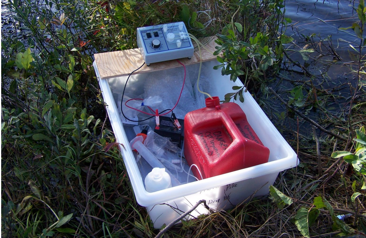
Figure 8.—Drip station used to treat the Stormy Lake outlet creek with rotenone.
