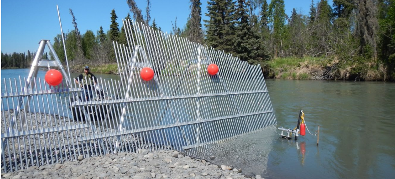
Figure 6.—Sonar coverage of the minor channel at the Kenai River RM 13.7 sonar site is achieved using an ARIS 1200 deployed on a tripod mount combined with a fixed weir.
