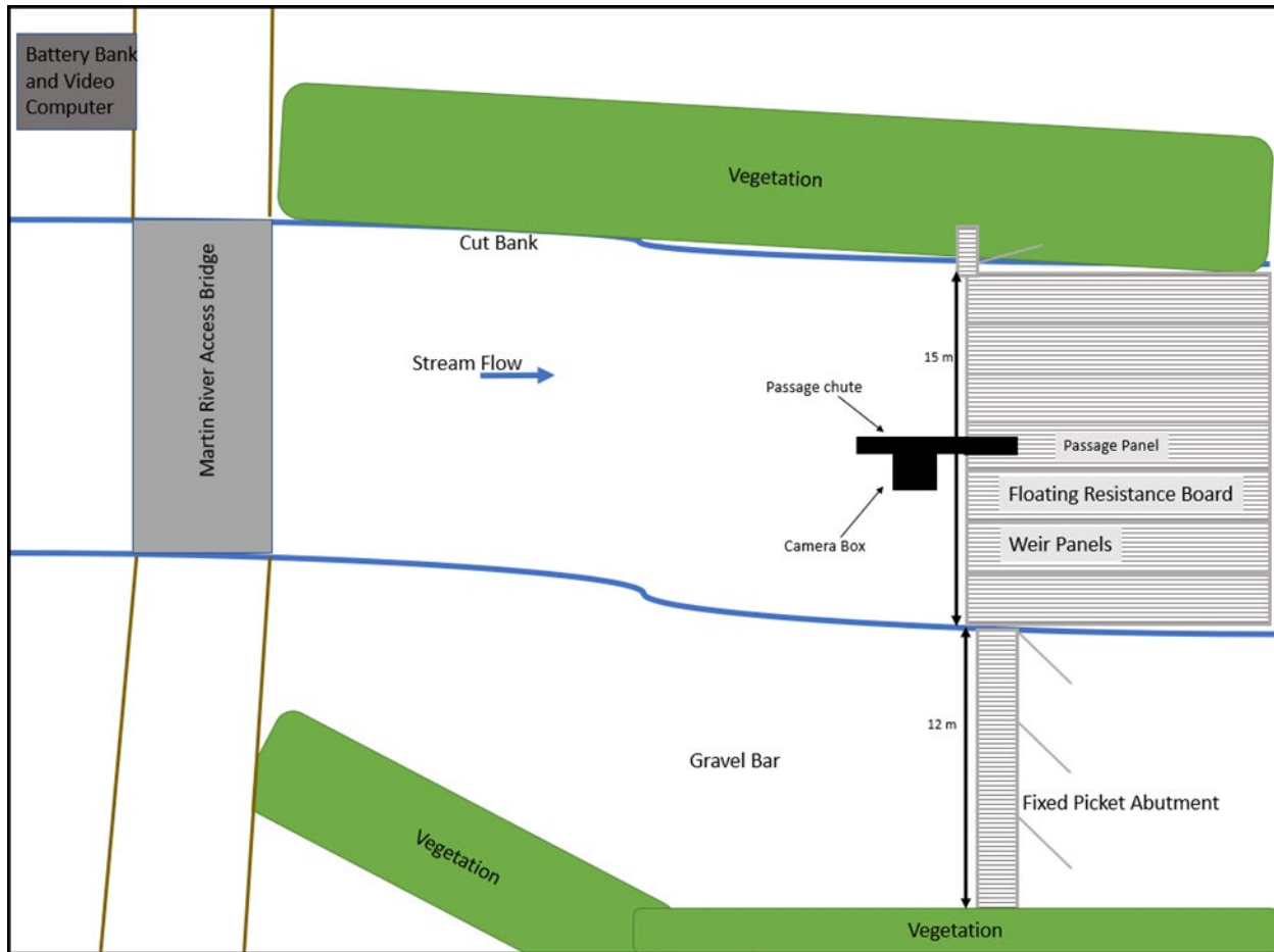
Figure 3.—Location and layout of the Battle Creek video weir in 2022.
