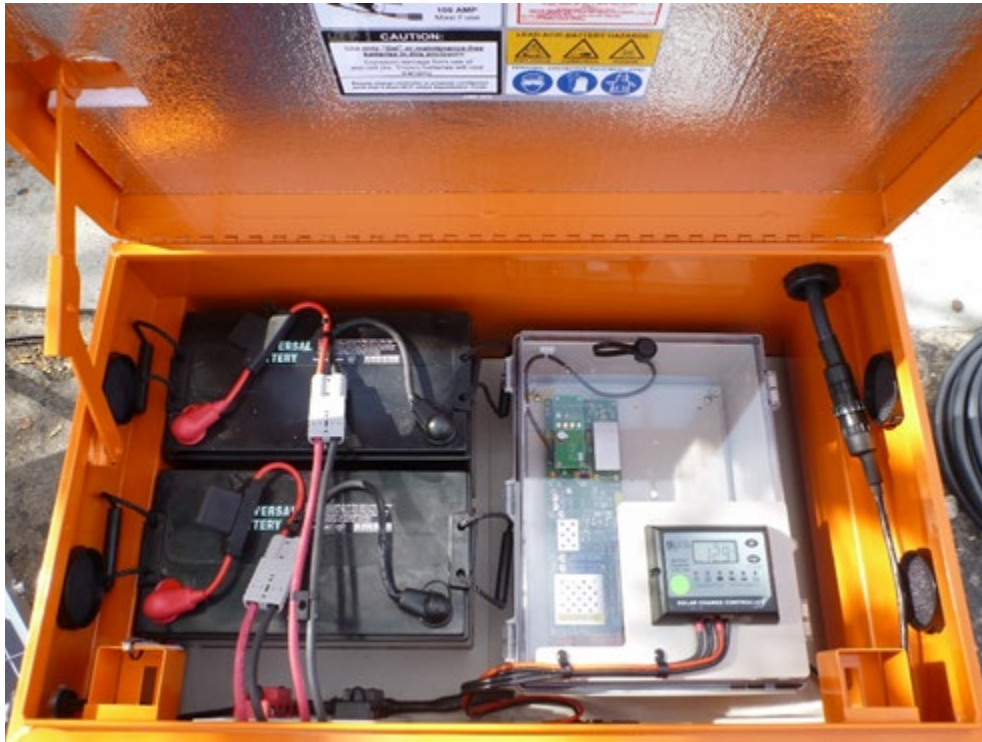
Figure A1-3.–Biomark IS 1001 chest enclosure showing the components and the 2 antenna exciter cables.
