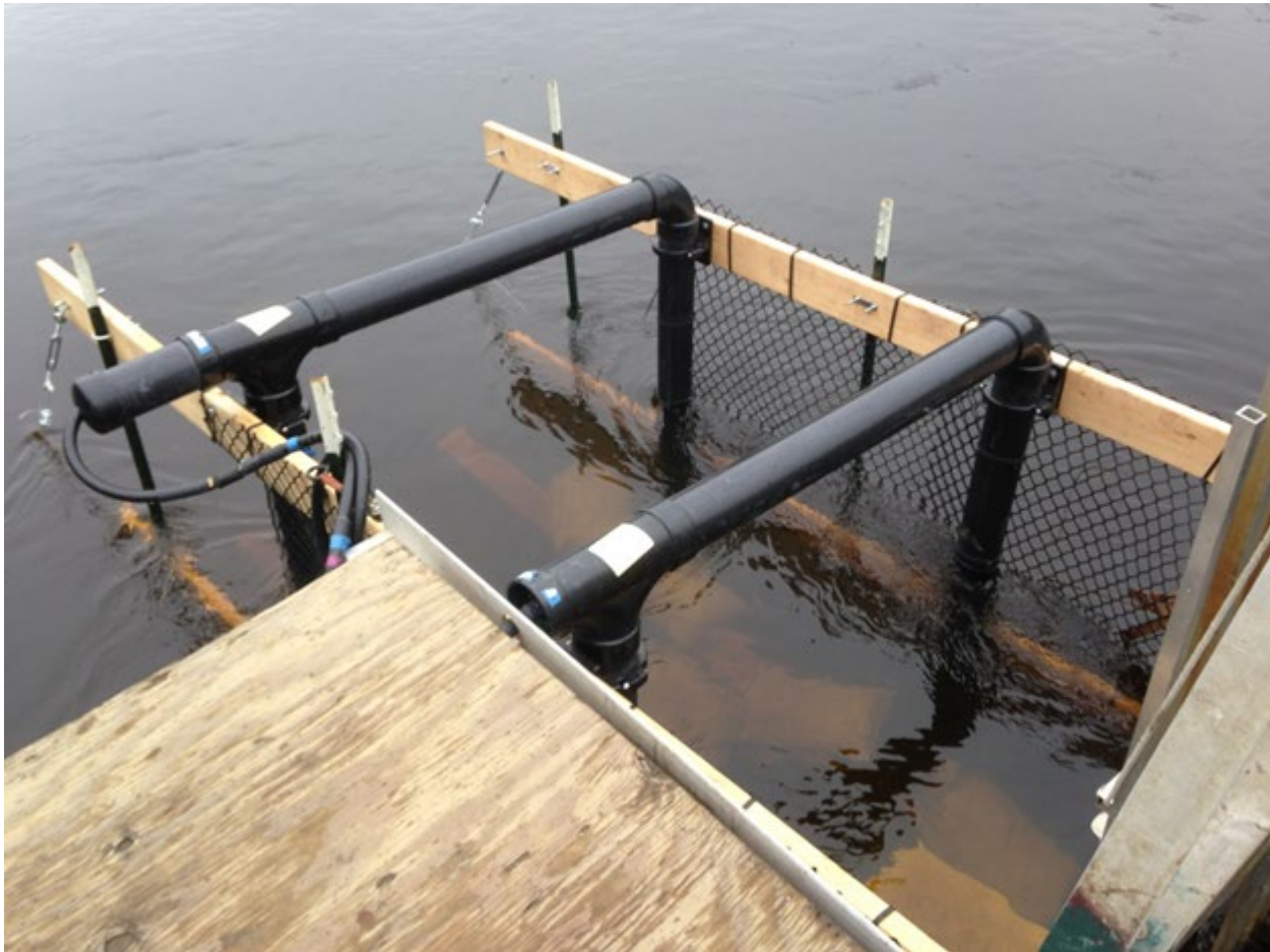
Figure A1-2.–PIT detection antennas above the Deshka River floating weir and cage, 2015.
