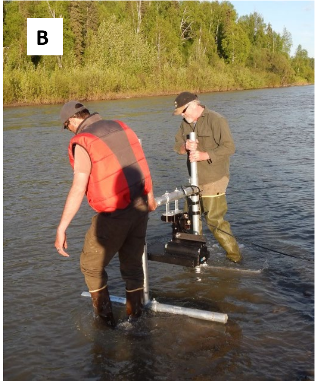
Figure 7.—An ARIS 1200 with a high-resolution lens mounted on a steel tripod for offshore deployment (A) and on an aluminum H-mount for nearshore deployment (B).
