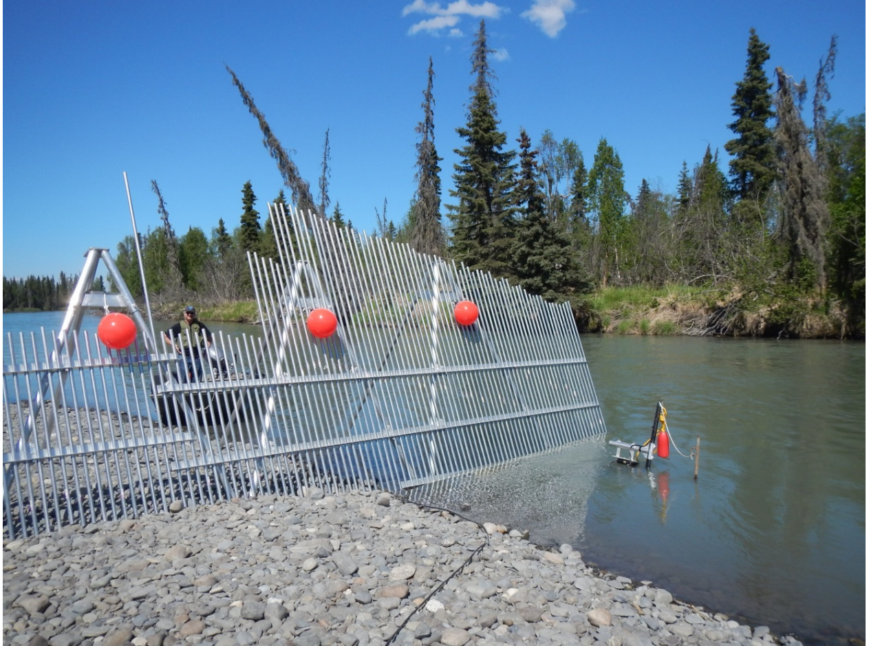
Figure 4.—Sonar coverage of the minor channel at the Kenai River RM 13.7 sonar site is achieved using an ARIS 1200 deployed on a tripod mount combined with a fixed weir.
