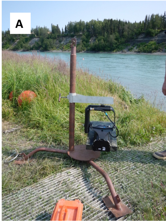
Figure 7.—An ARIS 1200 with a high-resolution lens mounted on a steel tripod for offshore deployment (A) and on an aluminum H-mount for nearshore deployment (B).
