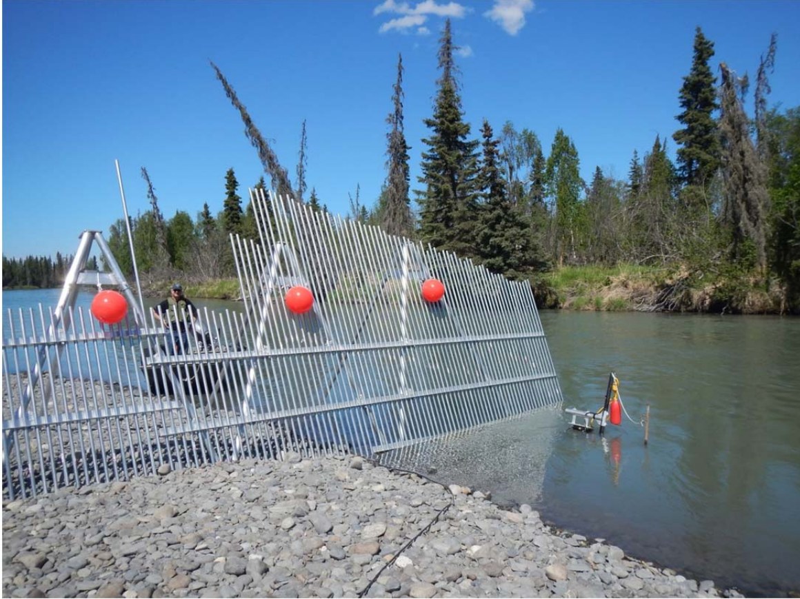
Figure 7.—Sonar coverage of the minor channel at the Kenai River RM 13.7 sonar site is achieved using an ARIS 1200 deployed on a tripod mount combined with a fixed weir.
