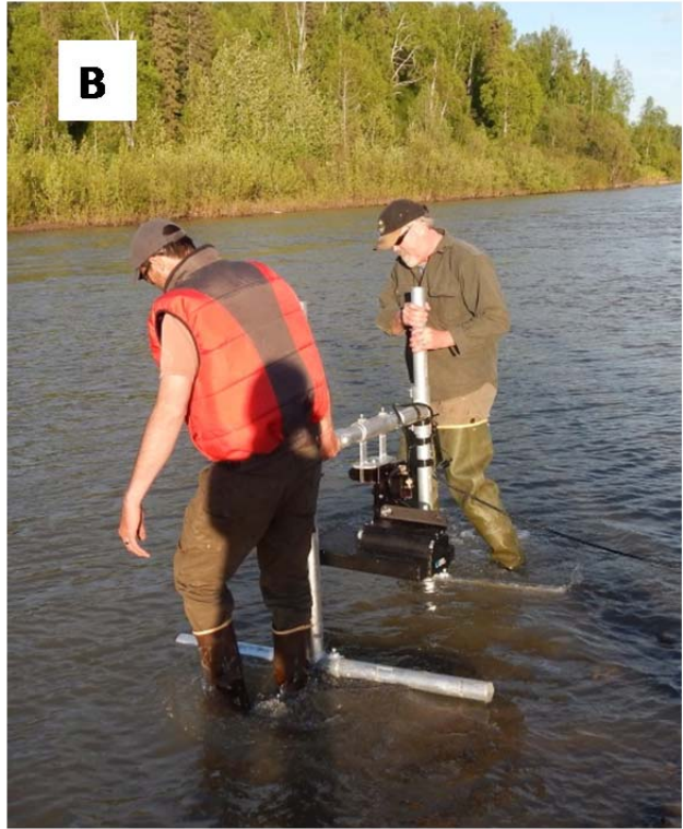
Figure 10.—An ARIS 1200 with a high-resolution lens mounted on a steel tripod for offshore deployment (A) and on an aluminum H-mount for near shore deployment (B).
