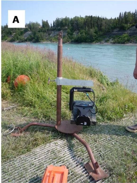
Figure 10.—An ARIS 1200 with a high-resolution lens mounted on a steel tripod for offshore deployment (A) and on an aluminum H-mount for near shore deployment (B).
