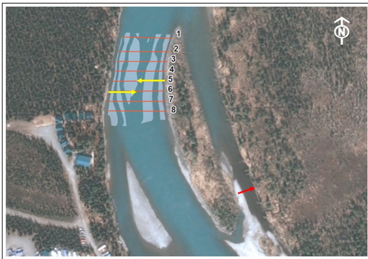
Figure 2.—Yellow arrows indicate preferred locations for sonars on each bank of the main channel. Note: Red arrow indicates approximate location for sonar in the minor channel.
