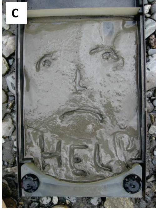
Figure 3. —A DIDSON-LR with a high-resolution lens (photos A and B). A silt-protection device is used (silt sock, photo B) to protect against silt build up in front of the lens (photo C).
