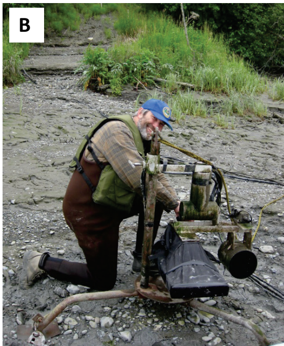
Figure 3. —A DIDSON-LR with a high-resolution lens (photos A and B). A silt-protection device is used (silt sock, photo B) to protect against silt build up in front of the lens (photo C).
