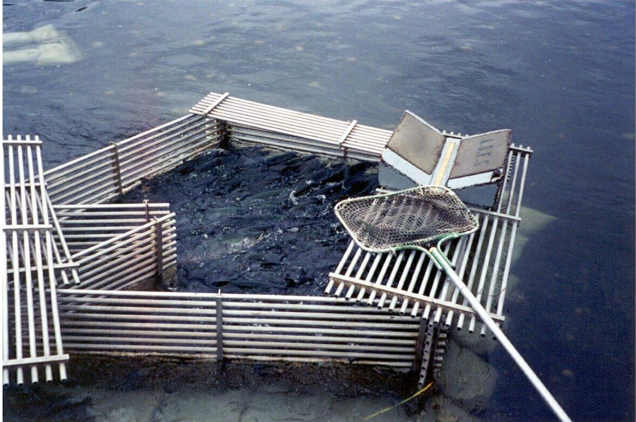
Figure 3.—The “Scott” 6-panel adult salmon live box trap (photo taken at Upper Station weir).
