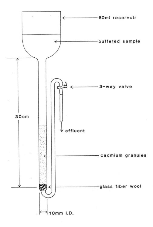
Figure 9.–Cadmium column used to reduce nitrate to nitrite in the manual analysis of nitrate + nitrite.
