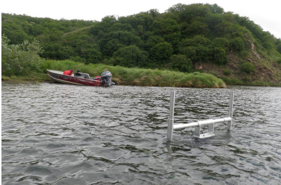
Figure 4.–Looking to the shore of the island at the sonar site. The H-mount is in the foreground.
