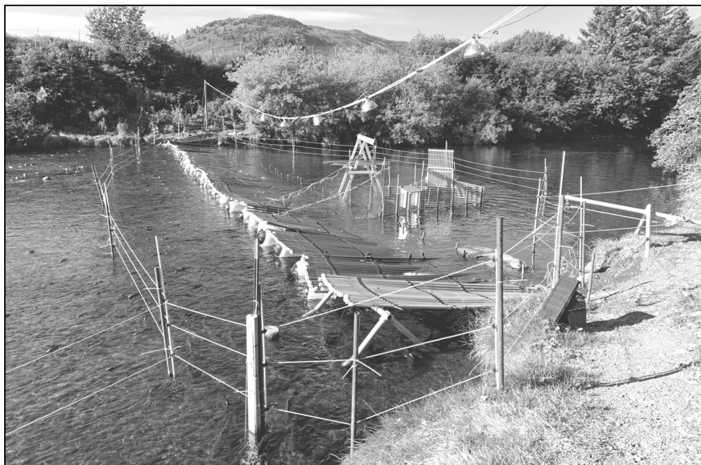
Figure 3.—Buskin River lower weir with counting gates and sampling trap.
