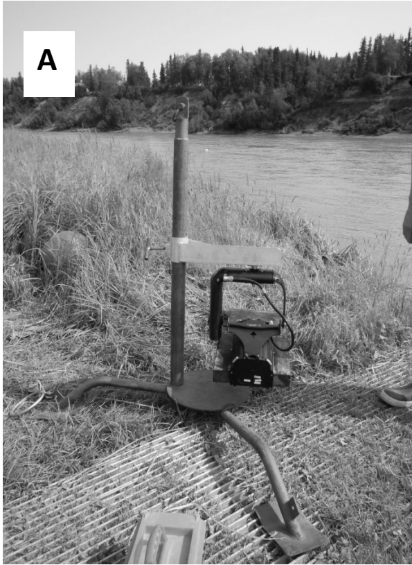
Figure 6.—An ARIS 1200 with a high-resolution lens mounted on a steel tripod for offshore deployment (A) and on an aluminum H-mount for nearshore deployment (B).
