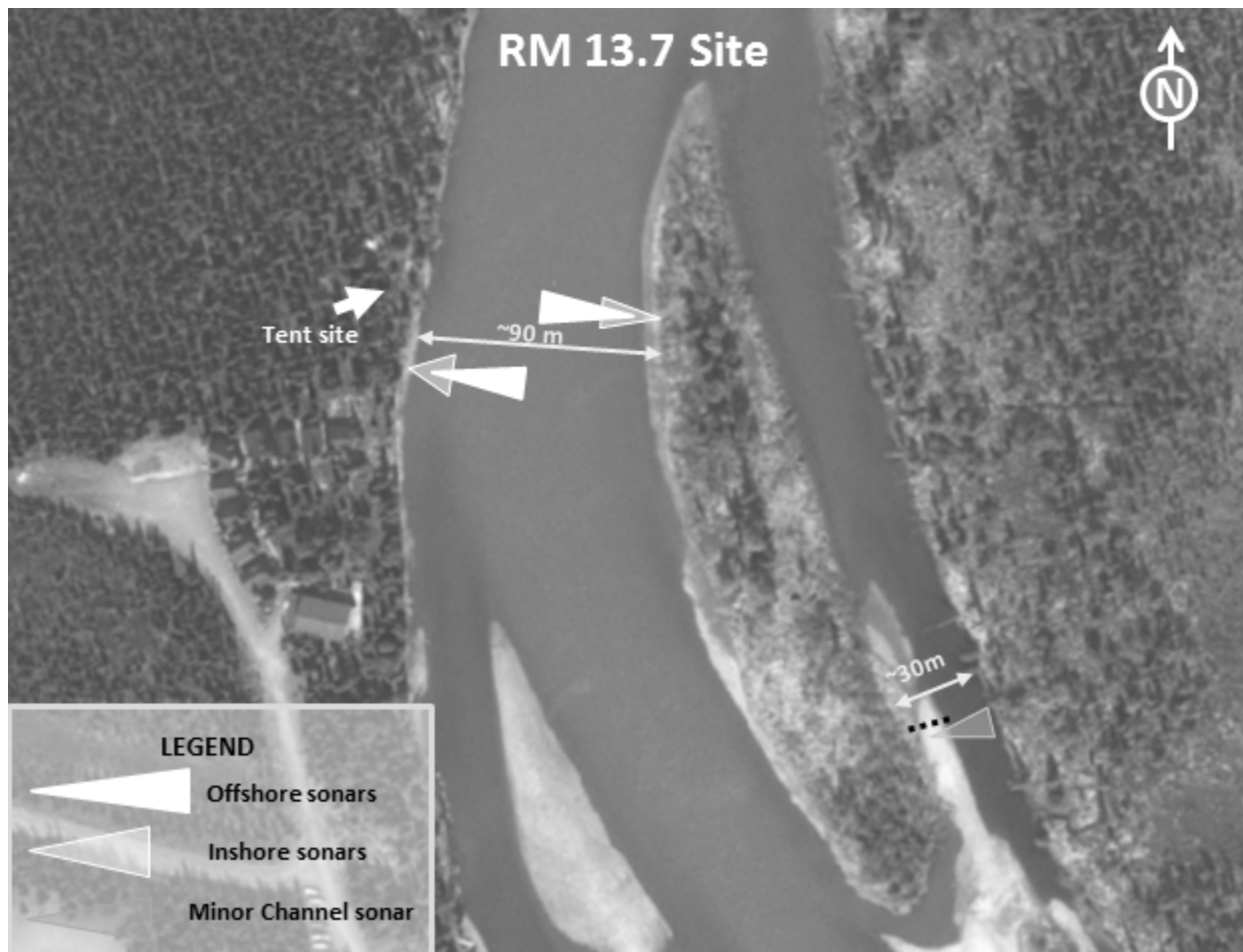
Figure 3.—Kenai River sonar site at river mile (RM) 13.7 showing approximate beam coverage. Note: Diagram is not to scale. Tent site indicates location where sonar electronics are housed. River flows north.
