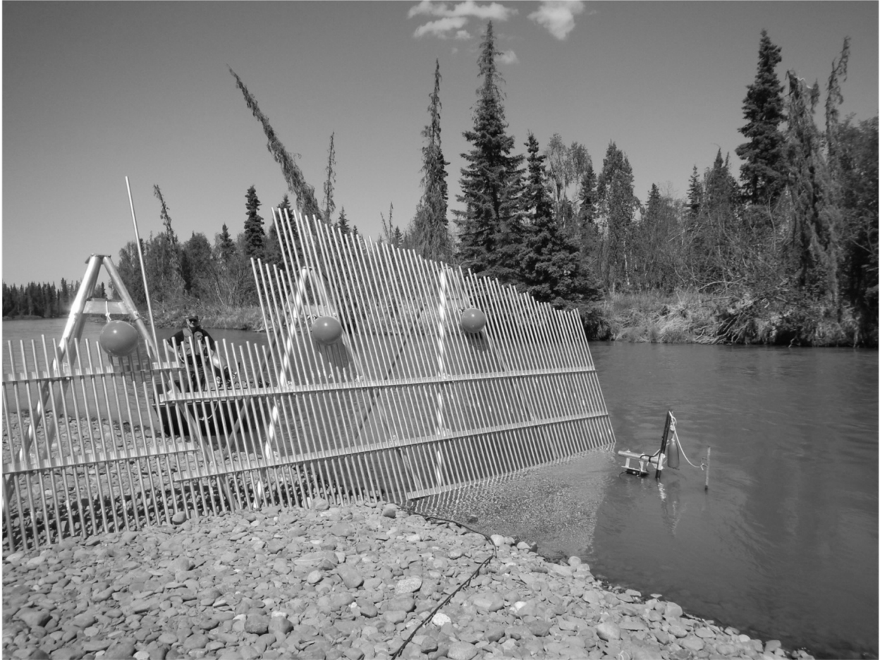
Figure 5.—Sonar coverage of the minor channel at the river mile (RM) 13.7 sonar site was achieved using an ARIS 1200 deployed on a tripod mount combined with a fixed weir.
