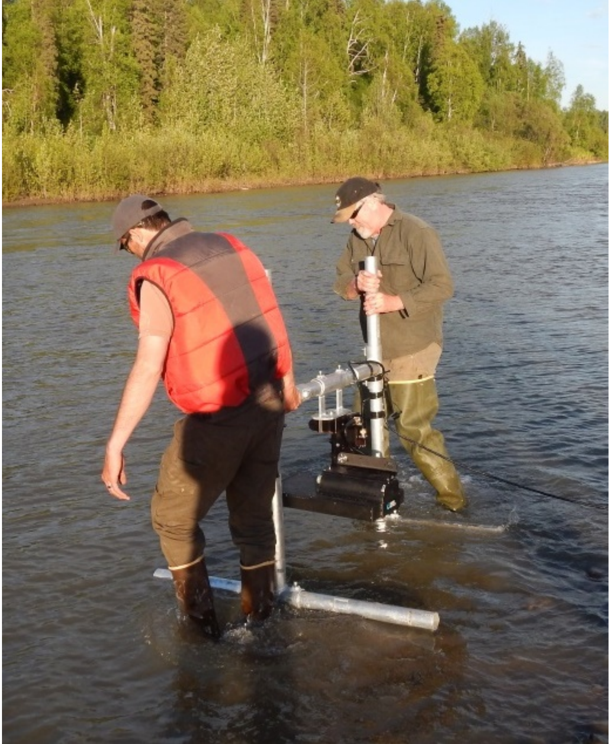
Figure 4.—ARIS mounted on an aluminum H-mount for nearshore deployment.
