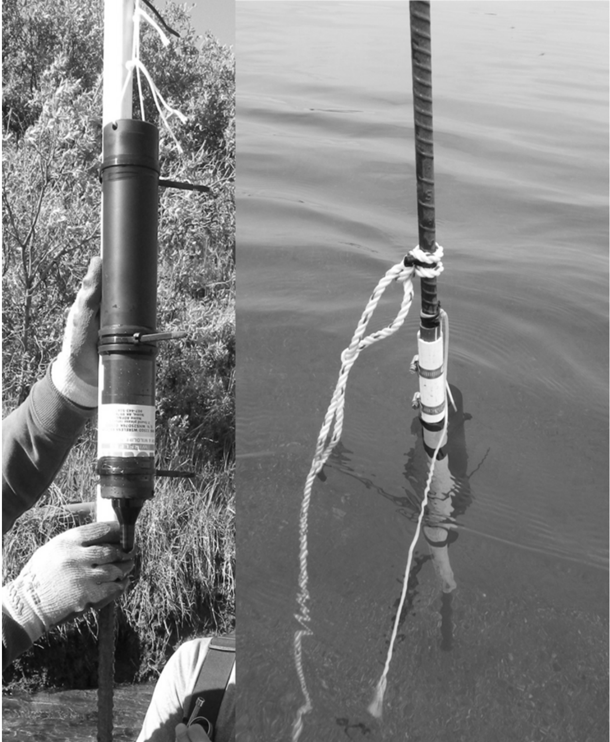
Figure 9.—River receiver setup and deployment.
