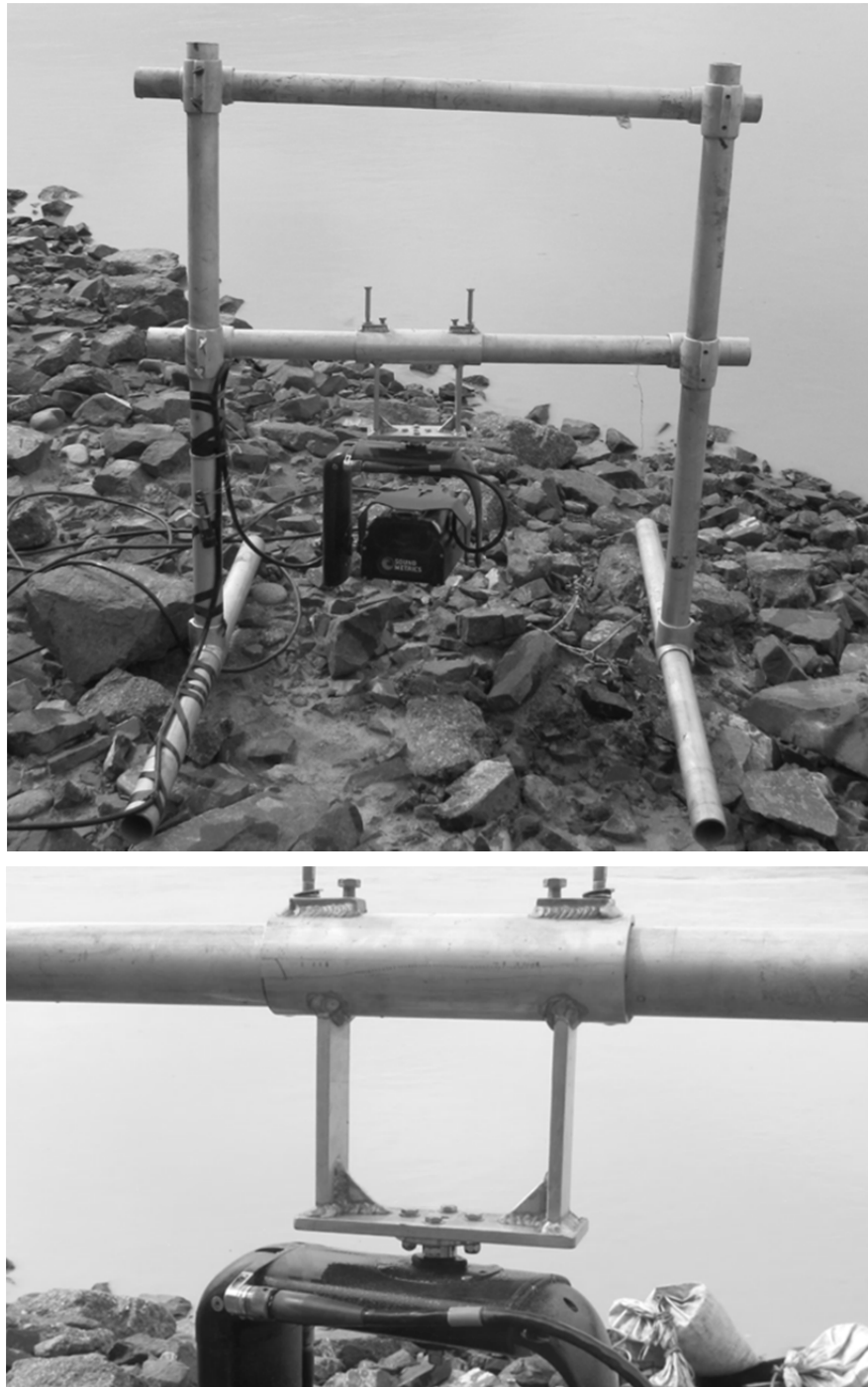
Figure 7.—View of ARIS imaging sonar and AR2 rotator mounted to an aluminum H mount (top), Close up view of mount for rotator (bottom), at the Eagle sonar project on the Yukon River, 2015.
