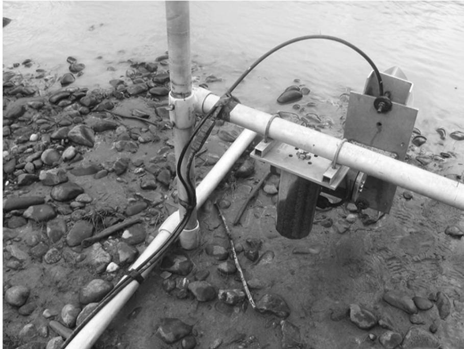
Figure 4.—Split-beam transducer mounted to an aluminum H-mount (top) and the same transducer mounted to 2 single-axis automated rotators (bottom), used on the left bank at the Eagle sonar project, on the Yukon River, 2015.
