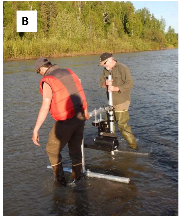
Figure 8.—An ARIS 1200 with a high-resolution lens mounted on a steel tripod for offshore deployment (A) and on an aluminum H-mount for nearshore deployment (B).
