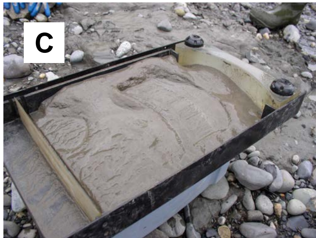
Figure 4.—A DIDSON-LR with a high-resolution lens is mounted on a steel tripod (photo A, top) and fitted with a custom fabric enclosure (photo B, middle), which protects against silt buildup in front of the lens (photo C, bottom).
