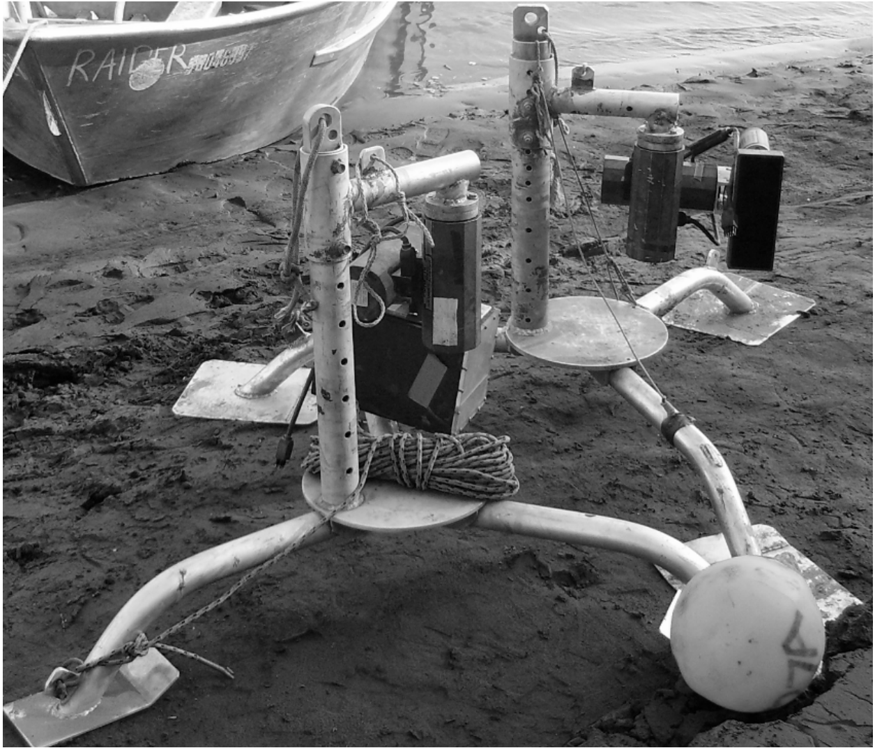
Figure 6.—DIDSON (front) and split-beam transducer mounted to pods with 662H dual axis rotators at the Pilot Station sonar project on the Yukon River.
