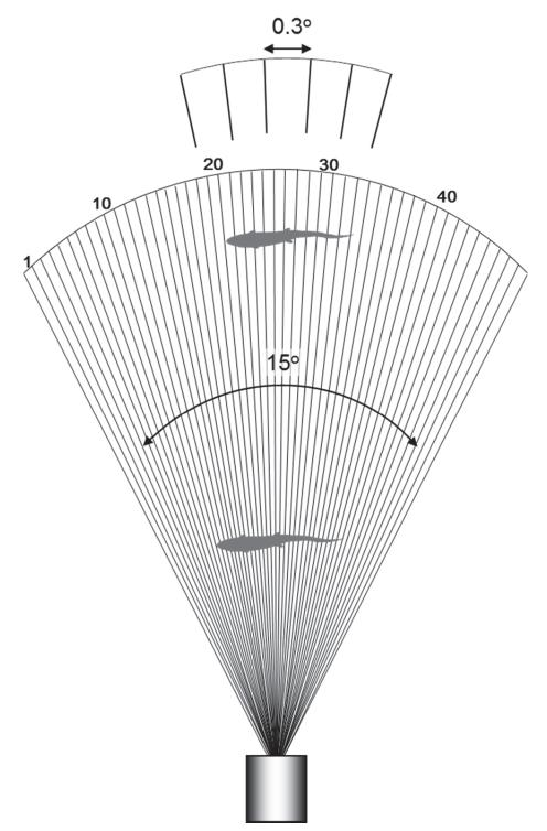
*Note:* because the beam widths grow wider with range, fish at close range are better resolved than fish at far range. *Note:* adapted from Burwen et al. 2007.
