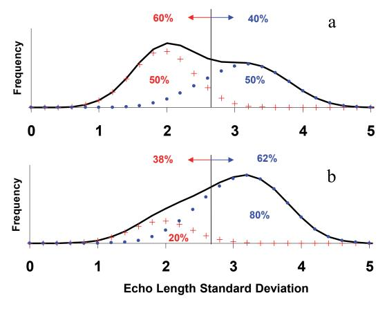
*Note:* Threshold-based discrimination is subject to bias when discriminating variables are imprecise. Solid lines are simulated frequency distributions of echo length standard deviation arising from component distributions due to sockeye salmon (plus symbols) and Chinook salmon (solid symbols).
