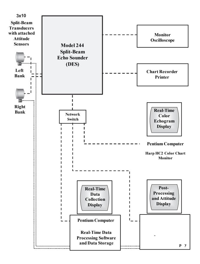
Figure 6.–Diagram of 2011 split-beam sonar system configuration and data flow.
