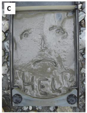
Figure 11.–DIDSON-LR with a high-resolution lens (on left in photos A and B) mounted next to a split-beam transducer (on right in photos A and B). A custom fit fabric enclosure shown in photo B protects against silt buildup in front of the lens as shown in photo C.
