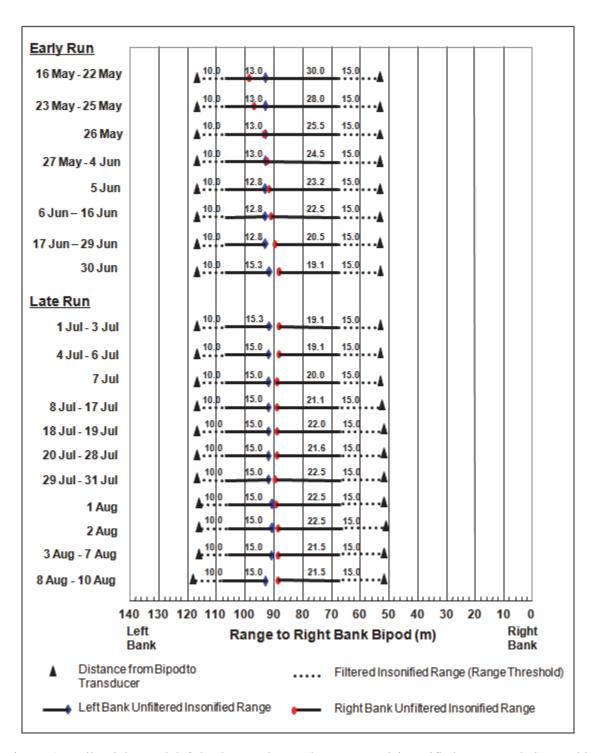
Figure 4.–Daily right- and left-bank transducer placement and insonified ranges relative to bipod tower located on the right bank, Kenai River RM 8.5, 2011.
