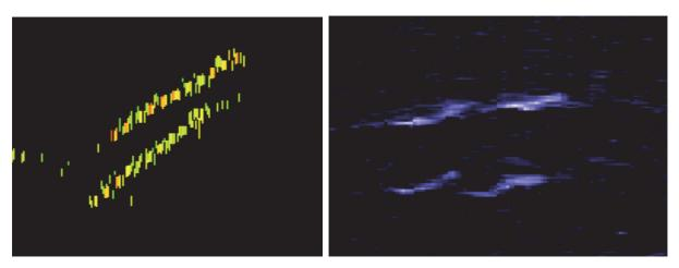
Figure 19.—Two pairs of small salmon swimming head-to-tail, as viewed on a split-beam echogram (left) and a DIDSON video frame (right).
