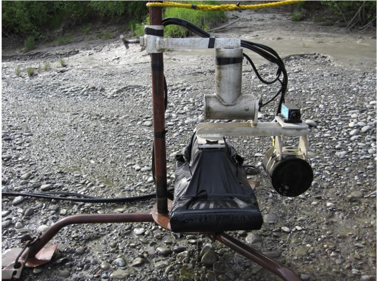
Figure 13.—A long-range DIDSON with a high-resolution large lens (left) is mounted side-by-side with a split-beam transducer (right). The DIDSON is sealed in a silt-proof enclosure.
