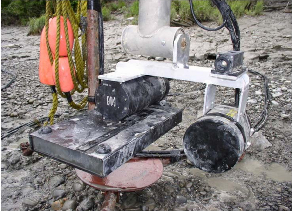
Figure 11.–Mounting system for a long-range, high resolution DIDSON (left on mount) and split-beam transducer (right on mount).
