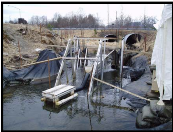
Figure 2.—Upstream view of incline-plane trap used to capture emigrant fish in Jordan Creek.
