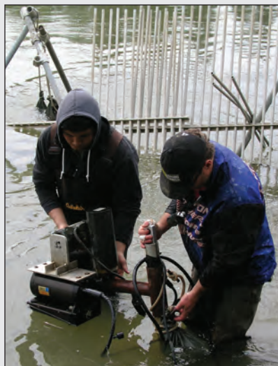
Sonar site technicians deploy two DIDSON transducers into the river each spring.
