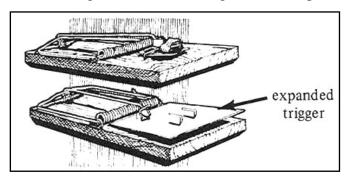
Figure H-12. Expanded trigger trap.
