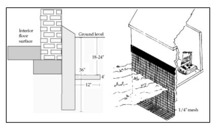
Figure H-8. Build curtain walls to keep rats out of buildings. Left: A curtain wall made of concrete that extends below ground level. Right: Wooden structures can be rodent-proofed by installing hardware cloth topped by a band of sheet metal.
