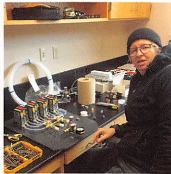
Dr. Amanda Kelley builds out an ocean acidification exposure system in the wet lab.
