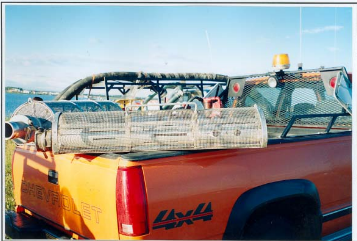
Figure 5. Photograph of First Generation Four-Inch Pump Water Intake Cylinder.
