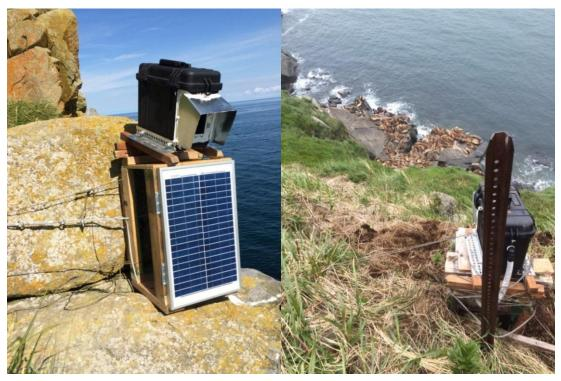
Figure 6. Self-contained DSLR camera system overlooking V3 fall-winter 2015–2016 and positioned above V1 Ledge fall-winter 2016–2017, Round Island, Alaska.
